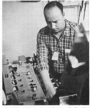
EXPOSED FILM is processed automatically after Don Fulton sets it up. A 100-ft. roll of 550 pictures is developed and printed in an hour and a half, with a foot and a half of film going through each minute. Because of the increased work volume in the Section, a new film processor has been ordered which will handle 50 ft. per minute.
